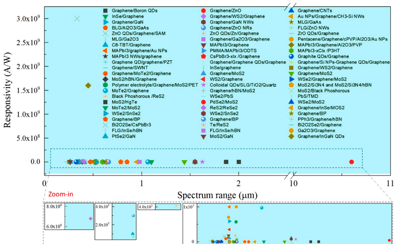
Fig. 7. Overview on responsivity of PDs using 2D heterostructures. Reproduced with permission from ref. [15] Copyright 2022 American Chemical Society.
