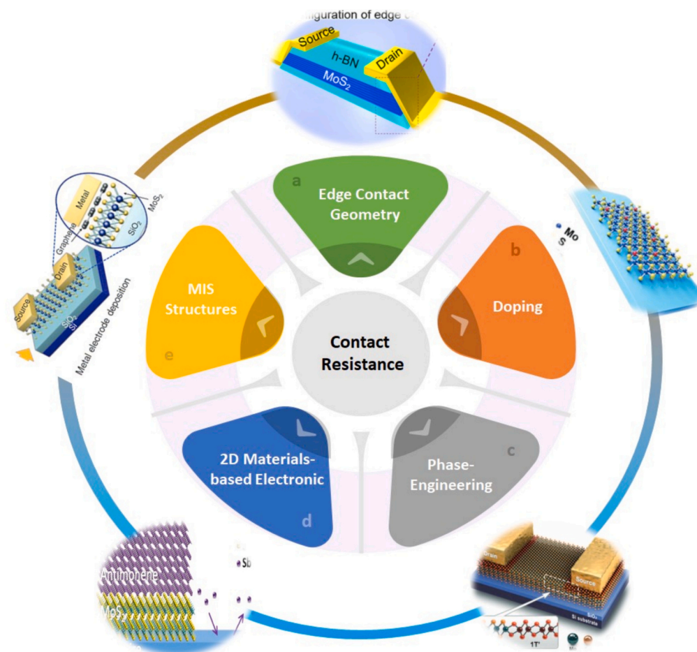
Fig. 10. Design strategies for IR PDs to diminish contact resistance. Inset: a. Edge-contacted hBN/MoS 2 /h-BN sandwich structure device. Reproduced with permission from ref. [239] Copyright 2019 American Chemical Society. b. Fe-doped monolayer MoS 2 device. Reproduced with permission from ref. [240] Copyright 2022 Wiley-VCH GmbH. c. A device with a 1 T'/2H phase homojunction of MoTe 2 . Reproduced with permission from ref. [241] Copyright 2015 American Association for the Advancement of Science. d. Transistor-based on a patterned MoS 2 on a sapphire substrate using \beta -antimonene as electrodes. Reproduced with permission from ref. [242] Copyright 2018 American Chemical Society. e. Schematic illustration of graphene interlayer inserted MoS 2 FETs with metal contacts. Reproduced with permission from ref. [243] Copyright 2018 Wiley-VCH GmbH.
